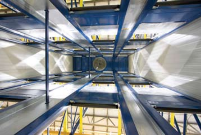
Looking up inside the vacuum chamber, where air is drawn through the pallet spacers and cases of products by the high powered fan placed at the top of each cell in the QFR Zone.
