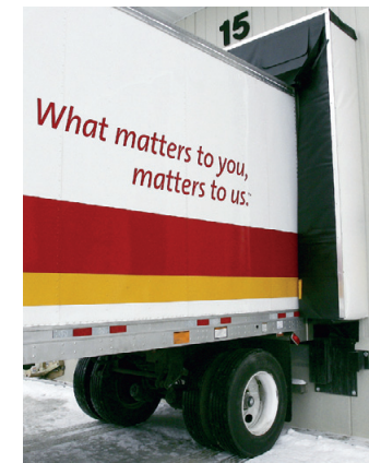
Dock doors that allow trucks to back up to the facility with the door still closed and sealed can reduce Biosecurity and tampering risks.
